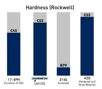
In Liquidmetal alloys, these properties are formed by the amorphous material composition. Additionally, no post mold processing is required to achieve final properties. Crystalline metals like 17-4 PH and 420 stainless steel require heat-treating to attain final properties, which can cause distortion, reduction of dimensional precision, and create quality problems if they are not processed correctly.
