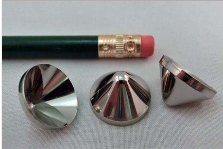
Fig. 15 As-moulded surface finish of Liquidmetal alloy parts
