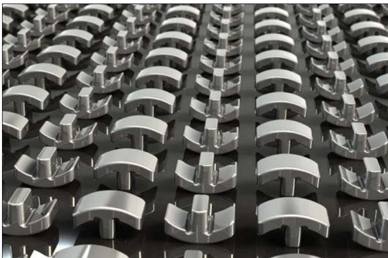
Fig. 7 Precise process and flow control allow small parts with high cavitation moulds to fill with high yields. This part was prototyped with 32 cavities and filled so well that the number of cavities could have been easily increased
