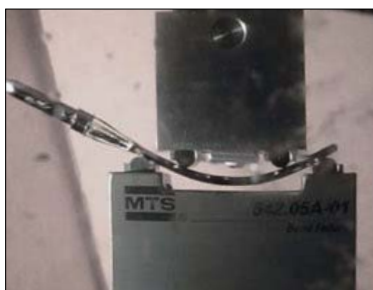
Fig. 3 Four-point bend test demonstrating the high elastic limit of Liquidmetal alloys. Test specimen is 45 mm long x 15 mm wide x 1.85 mm thick. This load represents 3% elastic strain, which is higher than the published strain limit of the material
