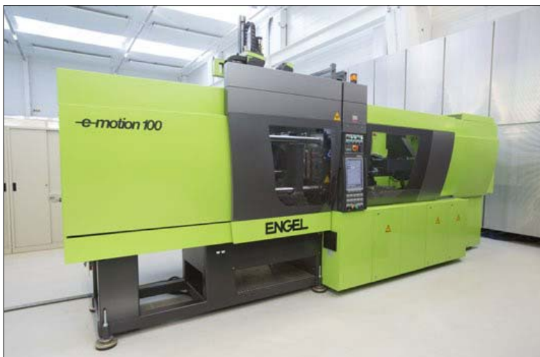
Fig. 6 Engel e-motion injection moulding machine for processing Liquidmetal alloys
