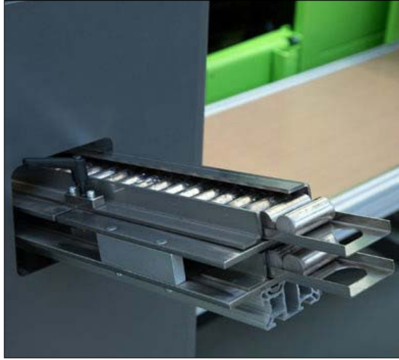
Fig. 8 Engel injection moulding machine alloy ingot loading magazine
