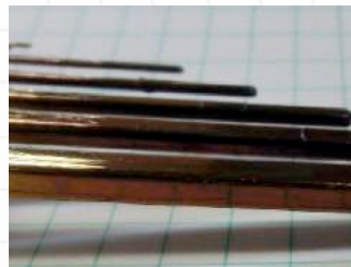
Figure 2: Illustration of color range that can be achieved with Liquidmetal's Mixed Oxide Finish. The L*a*b* color space values for the bright and dark ends of the spectrum are given. Darker colors are obtained by media blasting the parts before the Mixed Oxide Finish process is complete.
