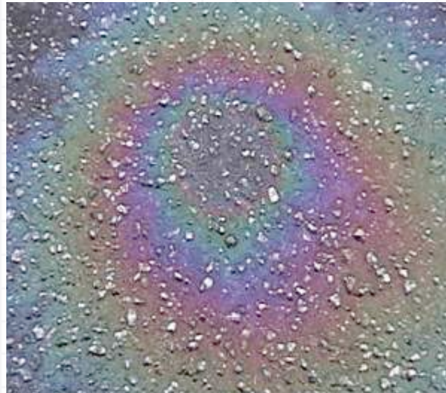
Figure 1: The thin film interference colors produced by water on oil are the same optical processes that create the Mixed Oxide Finish colors in Liquidmetal alloys
