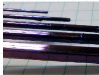
Figure 2: Illustration of color range that can be achieved with Liquidmetal's Mixed Oxide Finish. The L*a*b* color space values for the bright and dark ends of the spectrum are given. Darker colors are obtained by media blasting the parts before the Mixed Oxide Finish process is complete.
