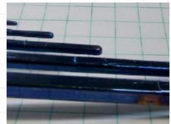
Figure 2: Illustration of color range that can be achieved with Liquidmetal's Mixed Oxide Finish. The L*a*b* color space values for the bright and dark ends of the spectrum are given. Darker colors are obtained by media blasting the parts before the Mixed Oxide Finish process is complete.
