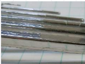
Figure 2: Illustration of color range that can be achieved with Liquidmetal's Mixed Oxide Finish. The L*a*b* color space values for the bright and dark ends of the spectrum are given. Darker colors are obtained by media blasting the parts before the Mixed Oxide Finish process is complete.
