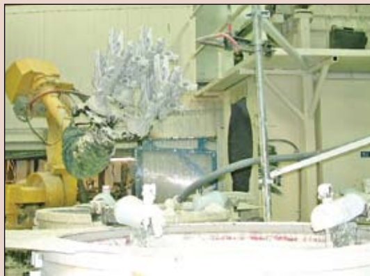
Signicast's rotating slurry wheel can accommodate the ever changing line of parts with just a few seconds of rotation.
