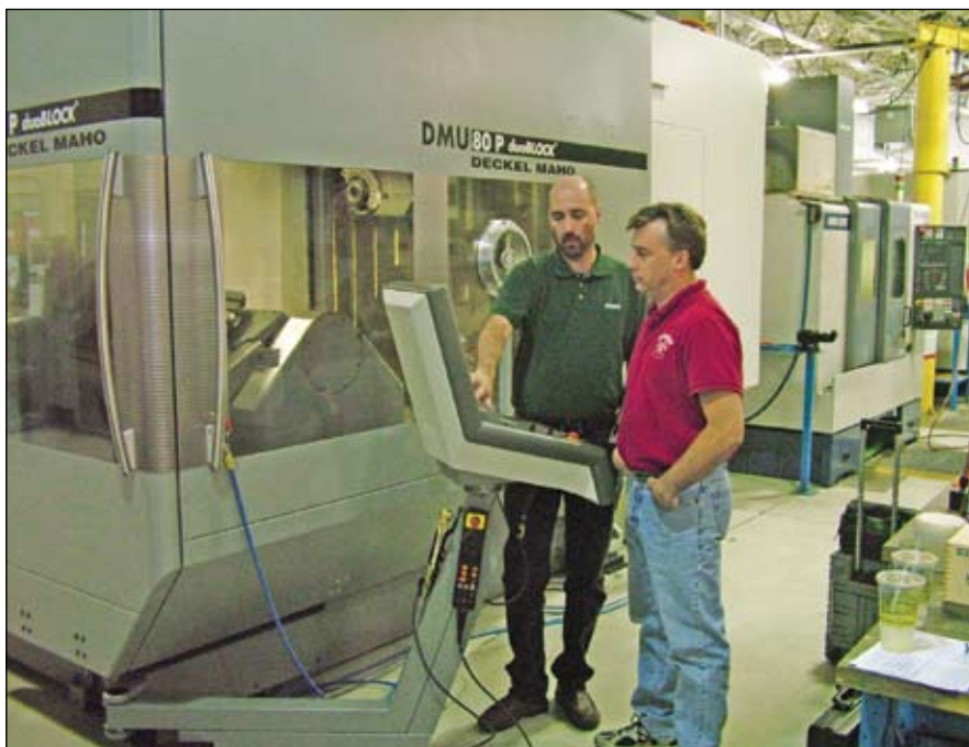
Signicast's 24/7 tooling department recently acquired this new five-axis CNC machine to increase its ability to build almost all of its tools in-house.
