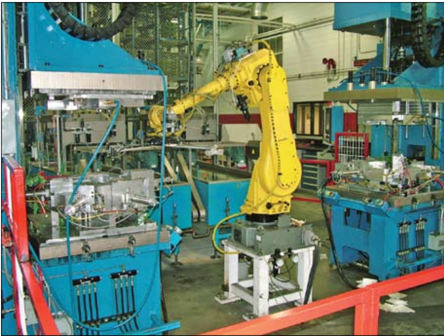
Robots inject wax into horizontal and vertical presses to create the molds. The wax is a tooth-paste-like consistency when injected, so there is less shrinkage as it hardens.
